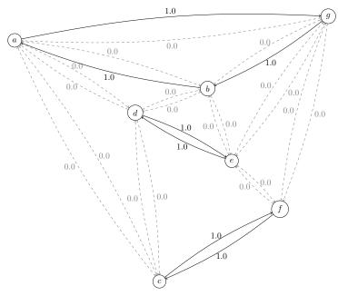
As it can be seen, there are tree disconnected sub-tours. Two of these include only two nodes. Forbidding sub-tours of size 2 is quite easy: in this case we only need to include the additional constraints:  $x_{(d,e)} + x_{(e,d)} \leq 1$  and  $x_{(c,f)} + x_{(f,c)} \leq 1$ .
